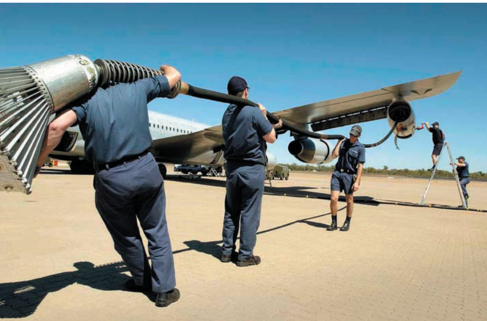
The hose and drogue system is more manpower intensive, as concerns routine maintenance. (PHOTO: RAAF)
