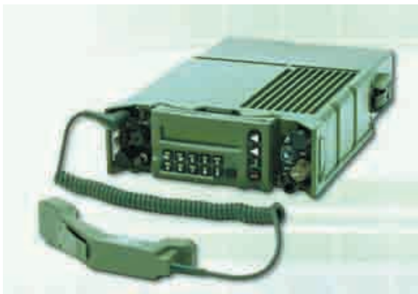
The CNR-2000 is an HF/VHF system available in either man-pack or vehicular mounted systems. (PHOTO: Selex)
