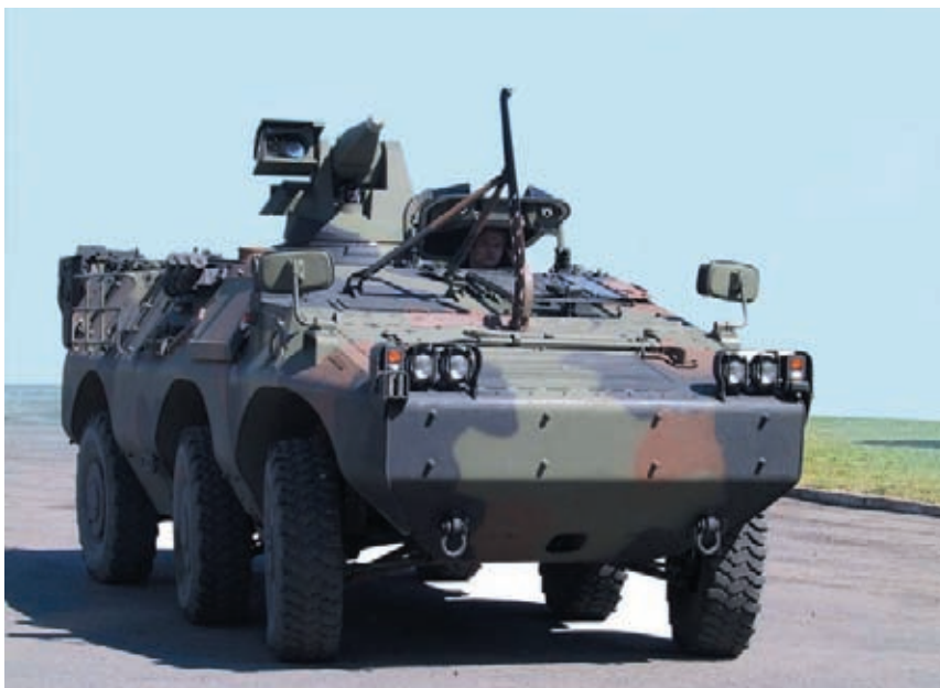
The 6x6 Puma seen outfitted with the 12.7mm HITROLE remote weapons station. (PHOTO: Finmeccanica)
