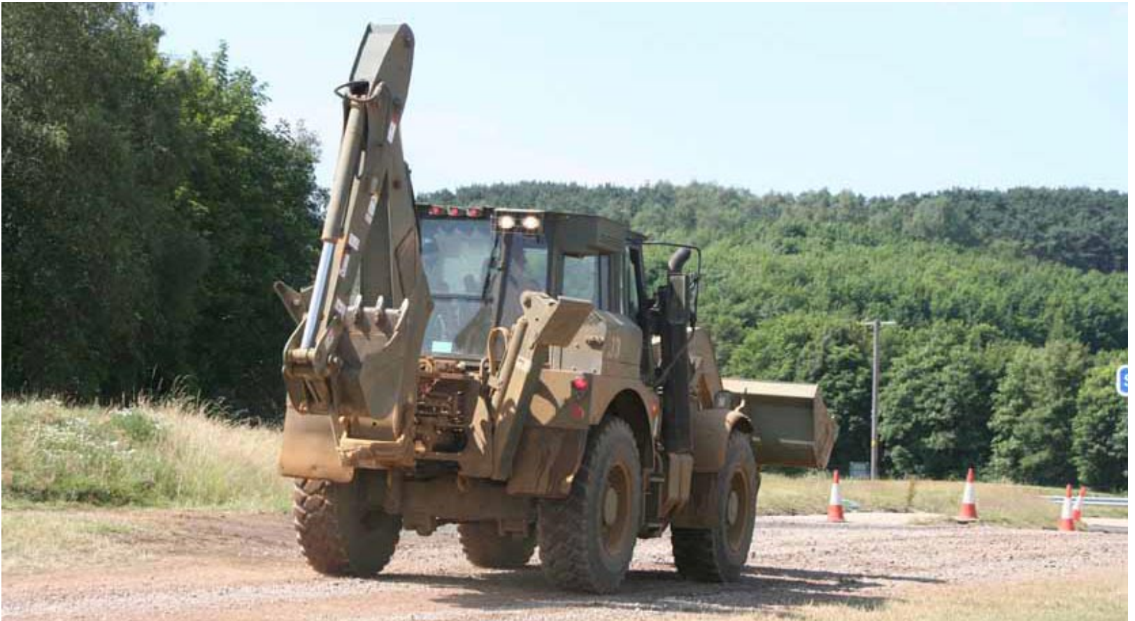
The militarised JCB 4cx backhoe loader, which in conjunction with the US Army, JCB has developed a high-speed backhoe called a High Speed Engineer Excavator (HMEE). (PHOTO: A. Baddeley)
