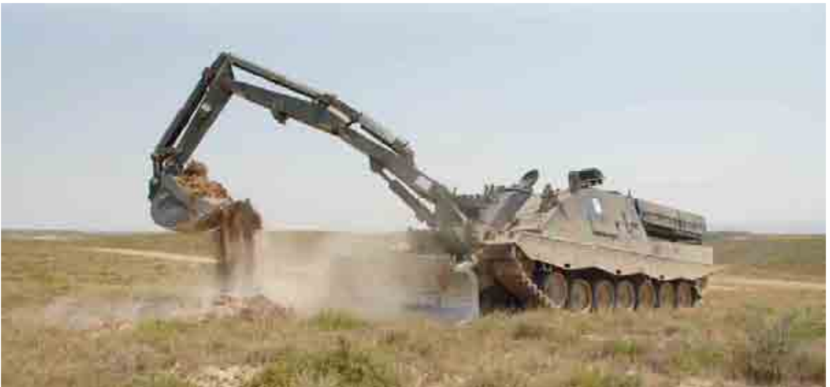
Rheinmetall's Kodiak AEV is based on the Leopard 2 chassis, and thus giving it clear potential for any existing Leopard users. (PHOTO: Rheinmetall)
